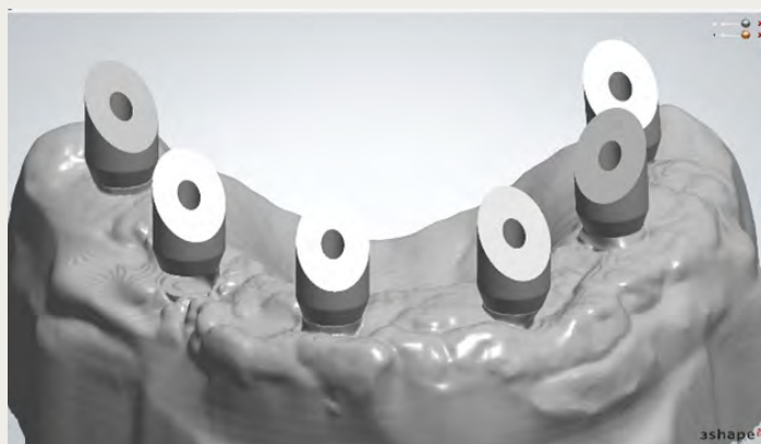
Fig. 1A: STL image of scan-bodies provide using photogrammetry (Micronmapper, S.I.N. Dental, USA)
