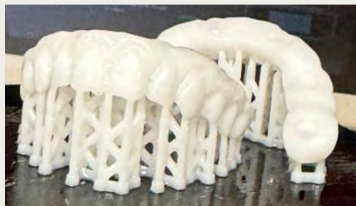
Fig. 2C: Prototype 3D printed (SprintRay Pro 55S, SprintRay, USA) using OnX Tough resin (SprintRay, USA).
