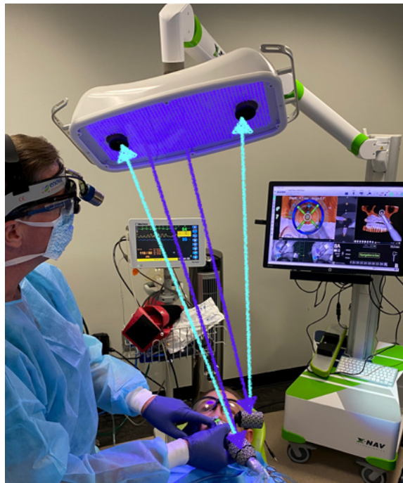
Light from the camera assembly bounces off the patient and handpiece tracking arrays back to the stereo cameras. The tracking system processes the images to give a live view of the surgical plan on the monitor.
